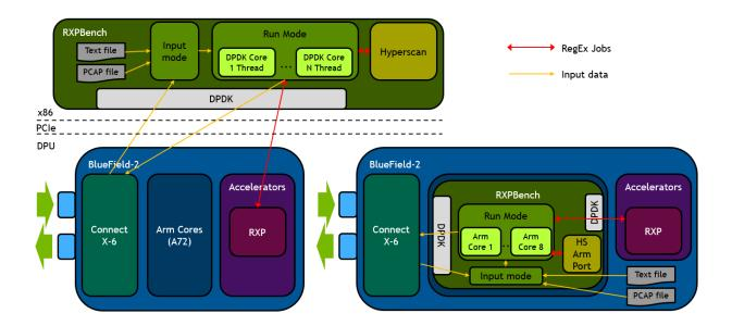
This diagram shows the relationship between RXPBench and the underlying BlueField-2 hardware when the application is being run on the x86 host (left side) or on the BlueField-2 Arm cores (right).
