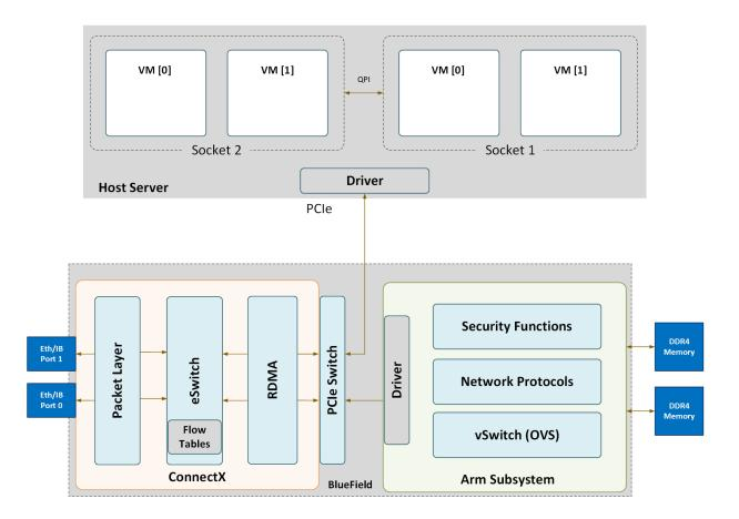
For each one of the BlueField DPU network ports, there are 2 physical PCIe networking functions exposed:
