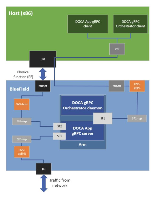
As can be seen above, the application is a bump-on-the-wire, and the gRPC-related traffic flows through a separate OVS bridge connected to the host using a virtual function (VF). More information about VFs and how to configure them can be found in the <u>NVIDIA DOCA Virtual</u> Functions User Guide.
