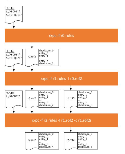
In this figure, r0.rules is the original ruleset or revision zero. This is compiled in the normal way resulting in r0.rof. The "[0-4]" class in rule ID two is then changed to "[0-9]" resulting in r1.rules (revision one). To incrementally update the RXPs rules memories for each new revision the incremental compile feature can be used. It can be seen that r1.rof2i is the result of incrementally compiling r1.rules using r0.rof2 as a baseline.
