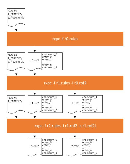
In this figure, r0.rules is the original ruleset or revision zero. This is compiled in the normal way resulting in r0.rof. The "[0-4]" class in rule ID two is then changed to "[0-9]" resulting in r1.rules (revision one). To incrementally update the RXPs rules memories for each new revision the incremental compile feature can be used. It can be seen that r1.rof2i is the result of incrementally compiling r1.rules using r0.rof2 as a baseline.
