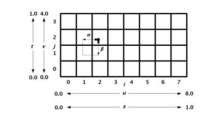
Figure 3.6. A texture image and the coordinates used to access it. This is a texture with  $w_t=8$  and  $h_t=4$ .  $\alpha$  and  $\beta$ , values used in blending adjacent texels to obtain a texture value, are also shown.
