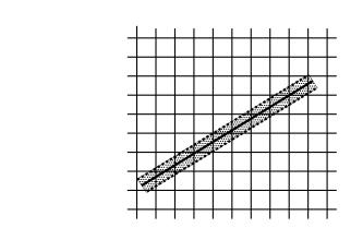
Figure 3.4. The region used in rasterizing a multisampled line segment (an x-major line segment is shown).
