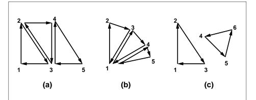
Figure 2.3. (a) A triangle strip. (b) A triangle fan. (c) Independent triangles. The numbers give the sequencing of the vertices in order within the vertex arrays. Note that in (a) and (b) triangle edge ordering is determined by the first triangle, while in (c) the order of each triangle's edges is independent of the other triangles.
