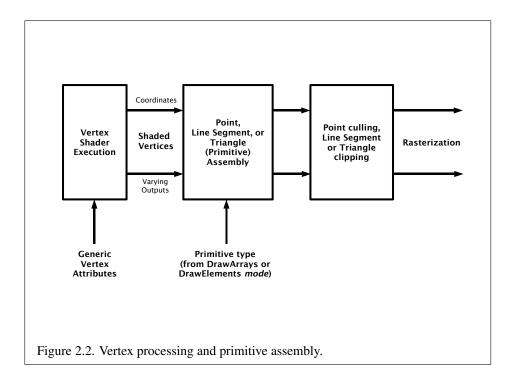
may insert new vertices into the primitive. The vertices defining a primitive to be rasterized have varying outputs associated with them.
