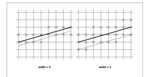
Figure 3.3. Rasterization of non-antialiased wide lines. x-major line segments are shown. The heavy line segment is the one specified to be rasterized; the light segment is the offset segment used for rasterization. x marks indicate the fragment centers produced by rasterization.
