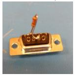
3) Now insert the **Female DB9 + Resistor** scheme in one of the port of **DB-9 Ribbon** scheme.
