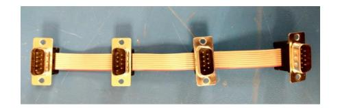
2) Take DB-9 Female connector. Solder short the following Pin group-1&2 and 7&8. Now Solder the 120ohm resistor across DB-9(1&2) & (7&8). Assemble the cap.
