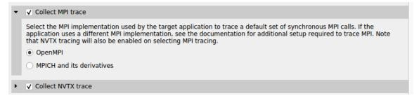
If you require more control over the list of traced APIs or if you are using a different MPI implementation, see github nvtx pmpi wrappers. You can use this documentation to generate a shared object to wrap a list of synchronous MPI APIs with NVTX using the MPI profiling interface (PMPI). If you set your LD\_PRELOAD environment variable to the path of that object, Nsight Systems will capture and report the MPI API trace information when NVTX tracing is enabled.
