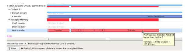
**HtoD transfer** indicates the CUDA kernel accessed managed memory that was residing on the host, so the kernel execution paused and transferred the data to the device. Heavy traffic here will incur performance penalties in CUDA kernels, so consider using manual cudaMemcpy operations from pinned host memory instead.
