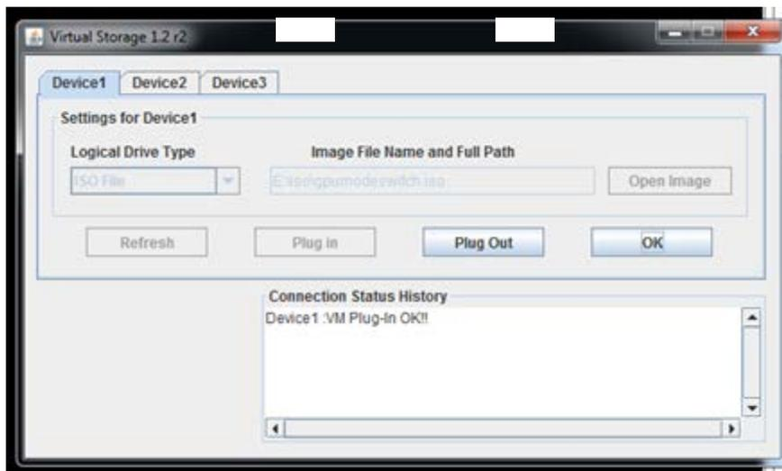
Figure 1 Connecting `gpumodeswitch.iso` via server remote management
