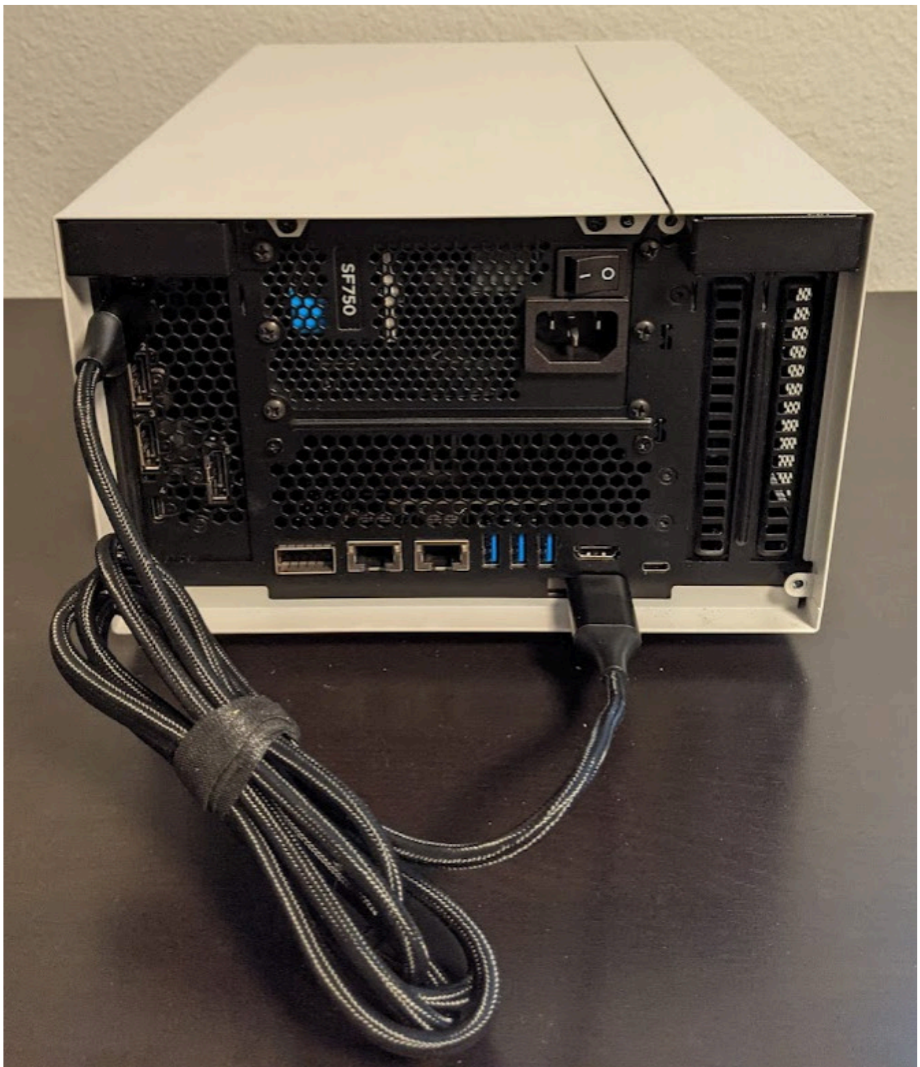
Fig. 24 DP-to-HDMI Cable Between GPU and Onboard HDMI Capture Card
