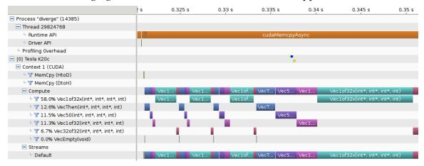
Along the top of the view is a horizontal ruler that shows elapsed time from the start of application profiling. Along the left of the view is a vertical ruler that describes what is being shown for each horizontal row of the timeline, and that contains various controls for the timeline. These controls are described in Timeline Controls
