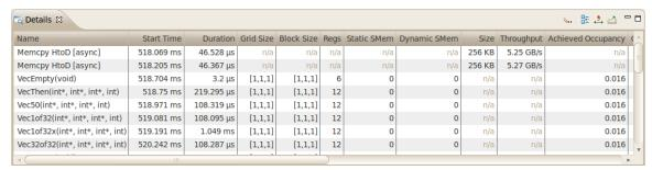
You can sort the data by column by left clicking on the column header, and you can rearrange the columns by left clicking on a column header and dragging it to its new location. If you select a row in the table, the corresponding interval will be selected in the Timeline View. Similarly, if you select a kernel or memcpy interval in the Timeline View the table will be scrolled to show the corresponding data.
