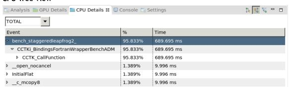
The CPU Details View displays a tree representing the application's execution on the CPU. Each node in the tree can represent a function called by the application. It shows the amount of time spent by the profiled application in the given function. The tree is organized to show the calling hierarchy among functions. The following modes are available:
