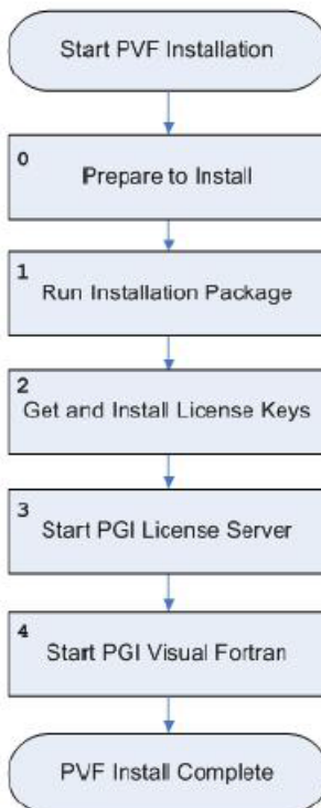
Figure 1 PVF Installation Overview
