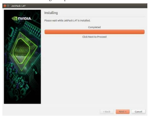
JetPack proceeds with setting up the Jetson Developer Kit target if the corresponding components were selected. For example, flashing the OS and pushing components to the Jetson Developer Kit target.
