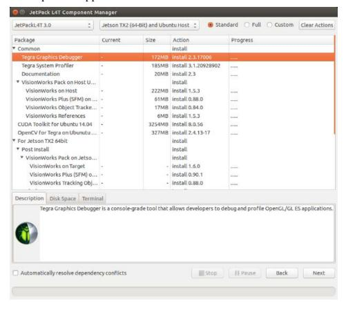
6. To run a standalone Ubuntu install, deselect Jetson target specific entries.
