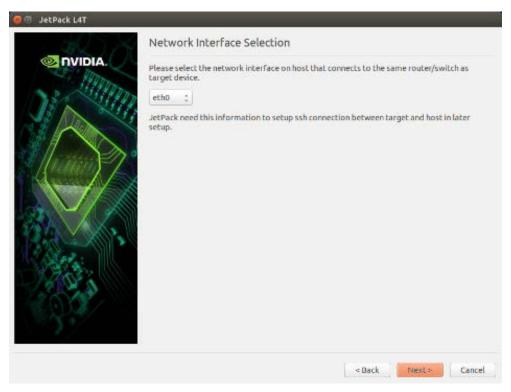
13. If you selected the Device get IP assigned by DHCP server on host and access **Internet via host machine** layout, you must select which interface to use for Internet access and which to use for the target interface.
