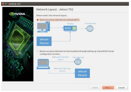
12. If you selected the Device access Internet via router/switch layout, you must select which interface to use for Internet access.
