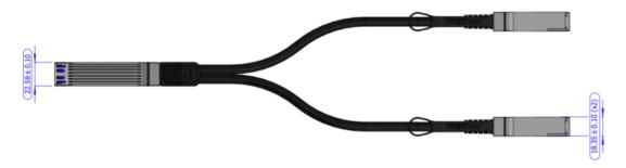
The splitting point is located at the head end, directly behind the strain relief.
