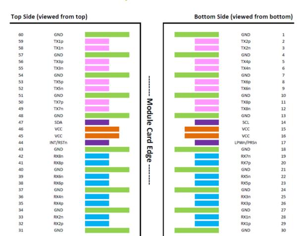
The Active Optical Cable (AOC) pin assignment is SFF-8679 compliant.
