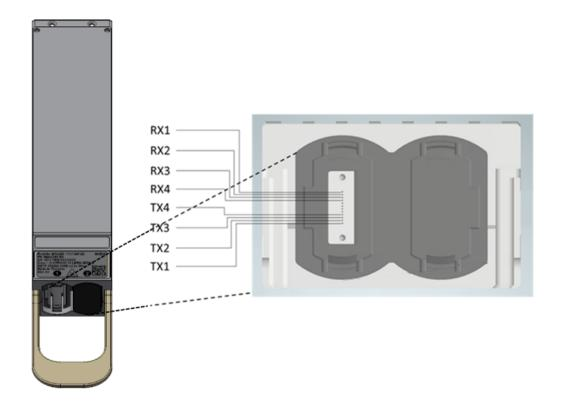
Module port labeling and lane routing. Txn/Rxn refers to the OSFP pin description
