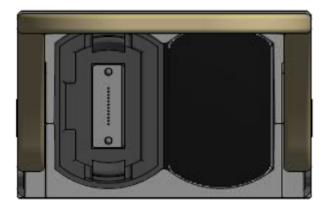
This is the 'head end'. The connectors in the 'tails' have same layout but only 2 transmit and 2 receive fibers with the middle 8 positions empty.
