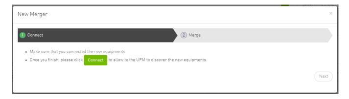
1. "Connect" Tab, it is important to physically connect the new equipment and confirm the connection. Then, click on a button which will open the boundary ports, change their state from Disabled to No-discover, and then deploy the active file again.
