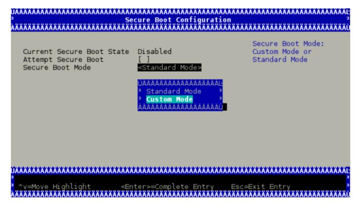
Once the platform is in "Custom Mode", a "Custom Secure Boot Options" menu entry appears which allows you to manipulate the UEFI database keys and certificates.
