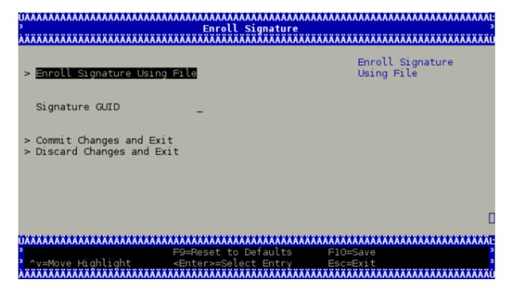
While enrolling the certificate file, you may enter a GUID along with the key certificate file. The GUID is the platform's way of identifying the key. It serves no purpose other than for you to tell which key is which when you delete it (it is not used at all in signature verification).
