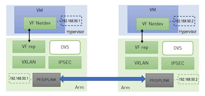
Support for strongSwan IPsec packet HW offload requires using VXLAN together with IPSec as shown here .
