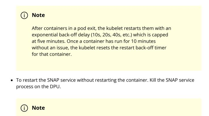
Restarting the SNAP service without restarting the container helps avoid the occurrence of back-off delays.
