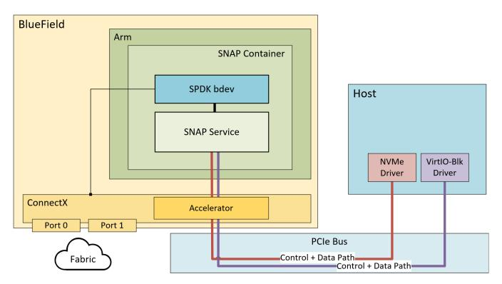
The traffic arriving from the host towards the emulated PCIe device is redirected to its matching storage controller opened on the mInx\_snap service.
