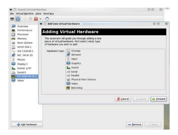
Choose a virtio-net device virtual function according to its PCIe device (e.g., 00:09.1), reboot or start the VM.
