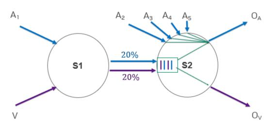
The diagram below shows an example of head of the line blocking scenario.
