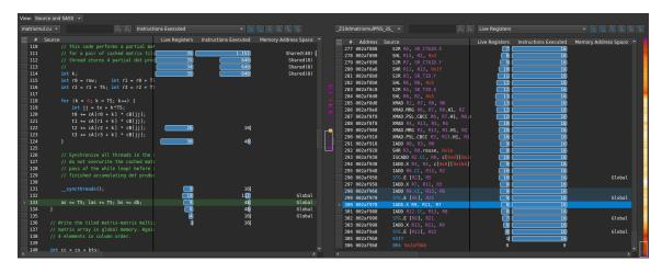
The *View* dropdown can be used to select different code (correlation) options. This includes SASS, PTX and Source (CUDA-C), as well as their combinations. Which options are available depends on the source information embedded into the executable.
