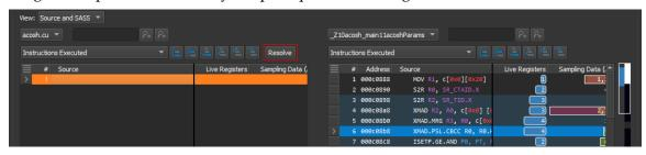
The heatmap on the right-hand side of each view can be used to quickly identify locations with high metric values of the currently selected metric in the dropdown. The heatmap uses a black-body radiation color scale where black denotes the lowest mapped value and white the highest, respectively. The current scale is shown when clicking and holding the heatmap with the right mouse button.
