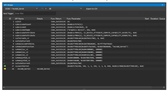
Use *Resume* (F5) and *Pause* to allow the program to run freely. Freeze control is available to define the behavior of threads currently not in focus, i.e. selected in the thread drop down. By default, the *API Stream* stops on any API call that returns an error code. This can be toggled in the *Debug* menu by *Break On API Error*.
