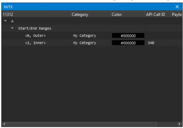
Use the *Current Thread* dropdown in the API Stream window to change the currently selected thread. NVIDIA Nsight Compute supports NVTX named resources, such as threads, CUDA devices, CUDA contexts, etc. If a resource is named using NVTX, the appropriate UI elements will be updated.
