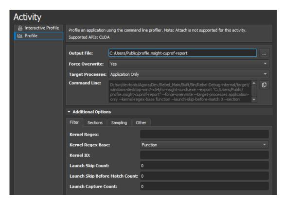
The *Section* tab allows you to select which sections should be collected for each kernel launch. Hover over a section to see its description as a tool-tip. To change the sections that are enabled by default, use the Sections/Rules Info tool window.
