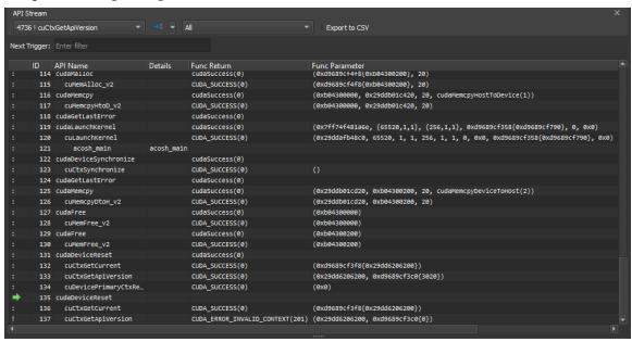
Whenever the target application is suspended, the window shows the history of API calls and traced kernel launches. The currently suspended API call or kernel launch (activity) is marked with a yellow arrow. If the suspension is at a subcall, the parent call is marked with a green arrow. The API call or kernel is suspended before being executed.
