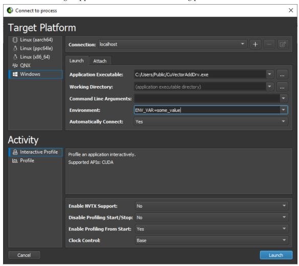
When using a remote platform, you will be asked to select or create a *Connection* in the top drop down. To create a new connection, select + and enter your connection details. When using the local platform, *localhost* will be selected as the default and no further connection settings are required. You can still create or select a remote connection, if profiling will be on a remote system of the same platform.
