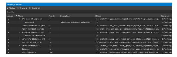
The enabled states of sections and rules are persisted across NVIDIA Nsight Compute launches. The *Reload* button reloads all sections and rules from disk again. If a new section or rule is found, it will be enabled if possible. If any errors occur while loading a rule, they will be listed in an extra entry with a warning icon and a description of the error.
