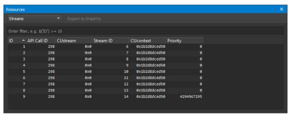
Using the dropdown on the top, different views can be selected, where each view is specific to one kind of resource (context, stream, kernel, ...). The *Filter* edit allows you to create filter expressions using the column headers of the currently selected resource.
