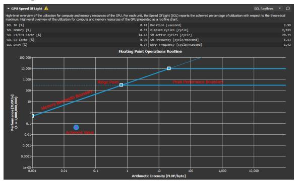
This chart actually shows two different rooflines. However, the following components can be identified for each:
