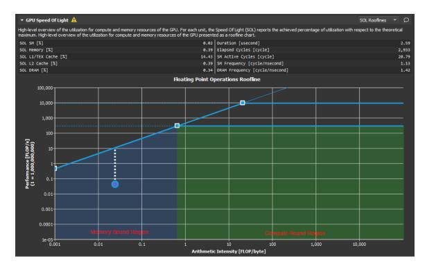
As shown here, the *ridge point* partitions the roofline chart into two regions. The area shaded in blue under the sloped *Memory Bandwidth Boundary* is the *Memory Bound* region, while the area shaded in green under the *Peak Performance Boundary* is the *Compute Bound* region. The region in which the *achieved value* falls, determines the current limiting factor of kernel performance.
