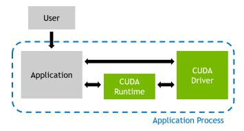
When profiling an application with NVIDIA Nsight Compute, the behavior is different. The user launches the NVIDIA Nsight Compute frontend (either the UI or the CLI)
