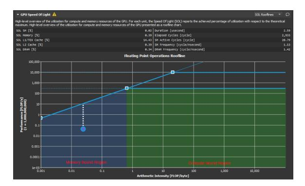
As shown here, the *ridge point* partitions the roofline chart into two regions. The area shaded in blue under the sloped *Memory Bandwidth Boundary* is the *Memory Bound* region, while the area shaded in green under the *Peak Performance Boundary* is the *Compute Bound* region. The region in which the *achieved value* falls, determines the current limiting factor of kernel performance.
