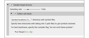
Nsight Systems can sample one process tree. Sampling here means interrupting each processor periodically. The sampling rate is defined in the project settings and is either 100Hz, 1KHz (default value), 2Khz, 4KHz, or 8KHz.
