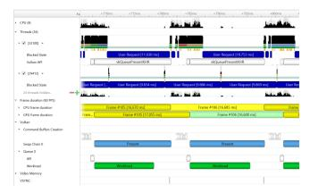
The Command Buffer Creation row displays time periods when command buffers were being created. This enables developers to improve their application's multi-threaded command buffer creation. Command buffer creation time period is measured between the call to **vkBeginCommandBuffer** and the call to **vkEndCommandBuffer**.
