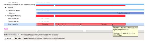
**HtoD transfer** indicates the CUDA kernel accessed managed memory that was residing on the host, so the kernel execution paused and transferred the data to the device. Heavy
