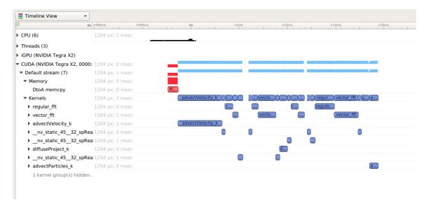
The easiest way to capture CUDA information is to launch the process from Nsight Systems, and it will setup the environment for you. To do so, simply set up a normal launch and select the **Collect CUDA trace** checkbox.
