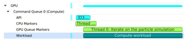
Detecting which CPU thread was blocked by a fence can be difficult in complex apps that run tens of CPU threads. The timeline view displays the 3 operations involved:
