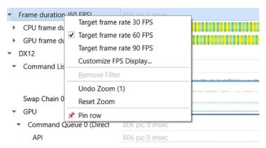
By clicking the Customize FPS Display option, a customization dialog pops up. In the dialog, you can now define the frame duration threshold to customize the view of the potentially problematic frames. In addition, you can define the threshold for the stutter analysis frames.
