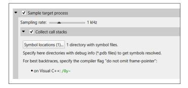
Nsight Systems can sample one process tree. Sampling here means interrupting each processor periodically. The sampling rate is defined in the project settings and is either 100Hz, 1KHz (default value), 2Khz, 4KHz, or 8KHz.
