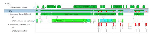
The Command List Creation row displays time periods when command lists were being created. This enables developers to improve their application's multithreaded command list creation. Command list creation time period is measured between the call to ID3D12GraphicsCommandList::Reset and the call to ID3D12GraphicsCommandList::Close.
