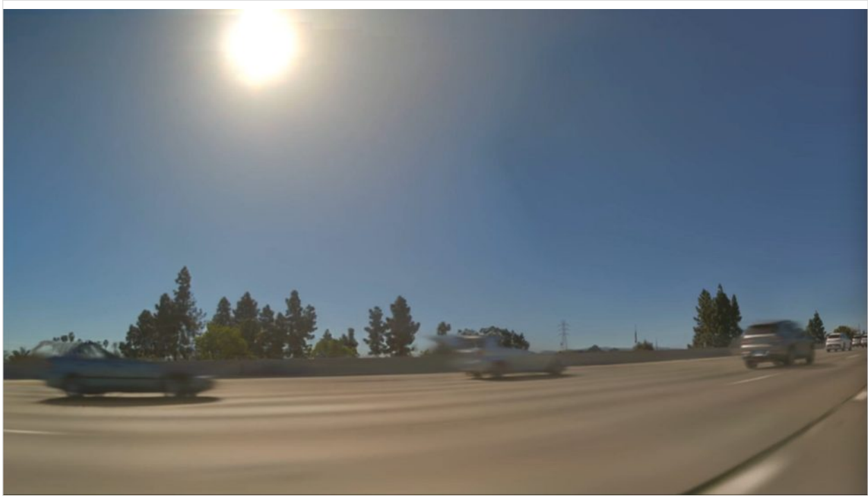
Figure 10a: Without LiDAR and camera orchestration, the vehicle of high speed is broken in the reconstruction
