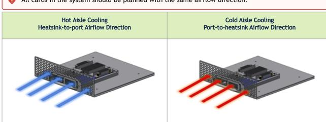
• All cards in the system should be planned with the same airflow direction.
