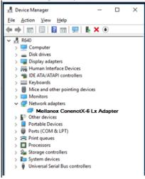
5. In the Value display box, check the fields VEN and DEV (fields are separated by '&'). In the display example above, notice the sub-string "PCI\VEN\_15B3&DEV\_1003": VEN is equal to 0x15B3 - this is the Vendor ID of NVIDIA Technologies; and DEV is equal to 1018 (for ConnectX-6 Lx) - this is a valid NVIDIA Technologies PCI Device ID.
