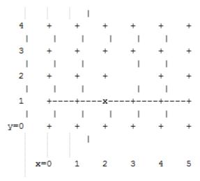
Assuming the dateline was between y=4 and y=0, this spanning tree has a branch that crosses a dateline. However, this cannot contribute to credit loops as it occurs on a 1D ring (the ring for x=3) that is broken by failure, as in the above example.
