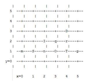
In a pristine fabric, torus-2QoS would generate the path from S to D as S-n-O-T-r-D. With failed switches O and T, torus-2QoS will generate the path S-n-I-q-r-D, with an illegal turn at switch I, and with hop I-q using a VL with bit 1 set. In contrast to the earlier examples, the second hop after the illegal turn, q-r, can be used to construct a credit loop encircling the failed switches.
