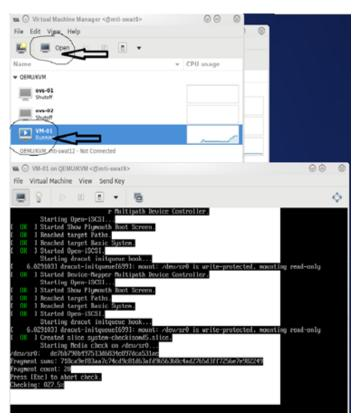
8. Follow the installation with "Minimal Install" and "Virtual Block Device" selection.
