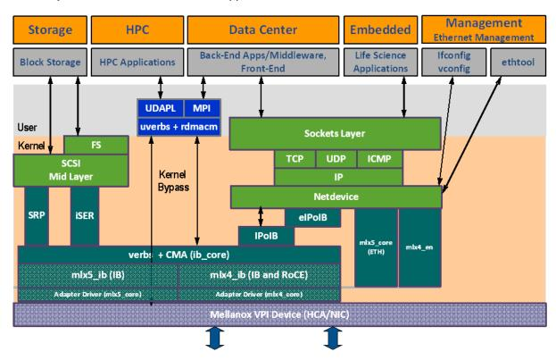
The following subsections briefly describe the various components of the NVIDIA OFED stack. mlx4 VPI Driver
