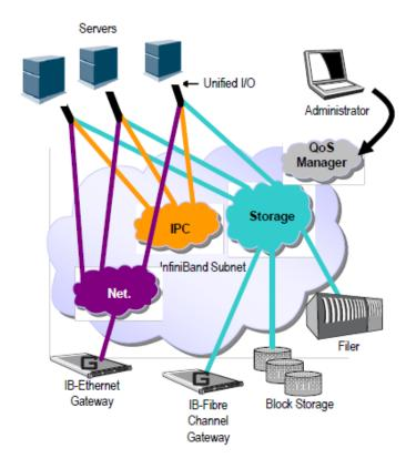
The basic need is to differentiate the service levels provided to different traffic flows, such that a policy can be enforced and can control each flow utilization of fabric resources. The InfiniBand Architecture Specification defines several hardware features and management interfaces for supporting QoS:
