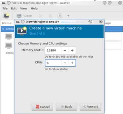
5. Create the disk image at the default root user location, for example: /var/lib/libvirt/images (NFS mount point). Make sure the storage is higher than 120GB and the virtual disk image is
