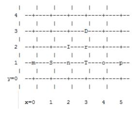
For a pristine fabric the path from S to D would be S-n-T-r-D. In the event that either link S-n or n-T has failed, torus-2QoS would use the path S-m-p-o-T-r-D.
