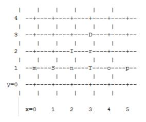
For a pristine fabric the path from S to D would be S-n-T-r-D. In the event that either link S-n or n-T has failed, torus-2QoS would use the path S-m-p-o-T-r-D.
