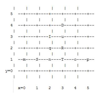
Suppose switches T and R have failed, and consider the path from S to D. Torus-2QoS will generate the path S-n-q-I-u-D, with an illegal turn at switch I, and with hop I-u using a VL with bit 1 set. As a further example, consider a case that torus-2QoS cannot route without deadlock: two failed switches adjacent in a dimension that is not the last dimension routed by DOR; here the failed switches are O and T:
