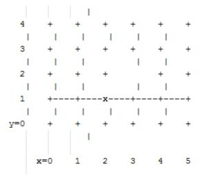
Assuming the dateline was between y=4 and y=0, this spanning tree has a branch that crosses a dateline. However, this cannot contribute to credit loops as it occurs on a 1D ring (the ring for x=3) that is broken by failure, as in the above example.
