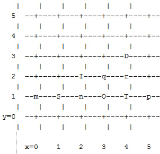
In a pristine fabric, torus-2QoS would generate the path from S to D as S-n-O-T-r-D. With failed switches O and T, torus-2QoS will generate the path S-n-l-q-r-D, with an illegal turn at switch I, and with hop l-q using a VL with bit 1 set. In contrast to the earlier examples, the second hop after the illegal turn, q-r, can be used to construct a credit loop encircling the failed switches.
