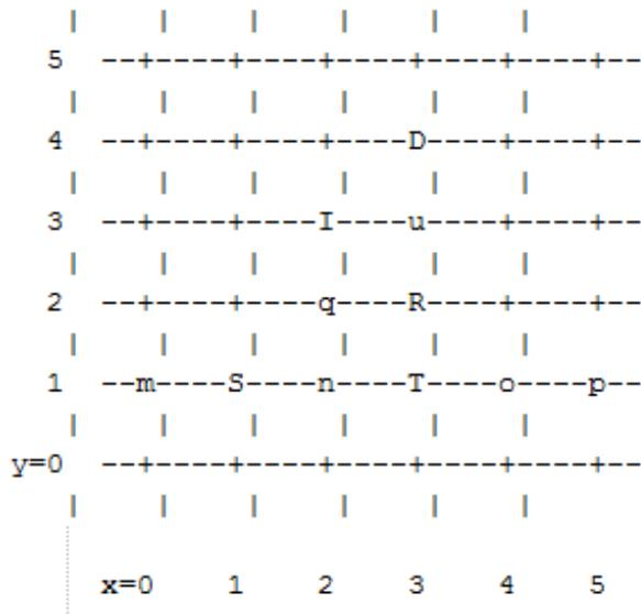
Suppose switches T and R have failed, and consider the path from S to D. Torus-2QoS will generate the path S-n-q-l-u-D, with an illegal turn at switch I, and with hop l-u using a VL with bit 1 set. As a further example, consider a case that torus-2QoS cannot route without deadlock: two failed switches adjacent in a dimension that is not the last dimension routed by DOR; here the failed switches are O and T:
