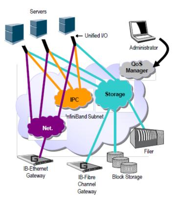
The basic need is to differentiate the service levels provided to different traffic flows, such that a policy can be enforced and can control each flow utilization of fabric resources. The InfiniBand Architecture Specification defines several hardware features and management interfaces for supporting QoS:
