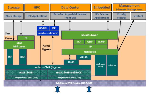
The following subsections briefly describe the various components of the NVIDIA OFED stack.
