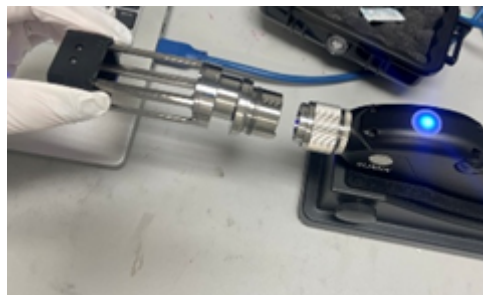
(a) Plugging the Quigon Tip (b) Plugging the ELSFP Cage Tip
