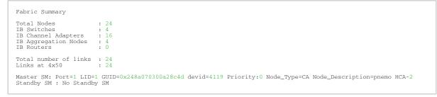
Check summary table in ibdiagnet output for errors in SHARP diagnostics stage. For example:
