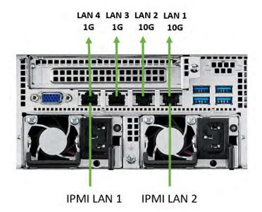
e. Use the following IPMI command to remote access serial console (user and password should be "admin" by default).
