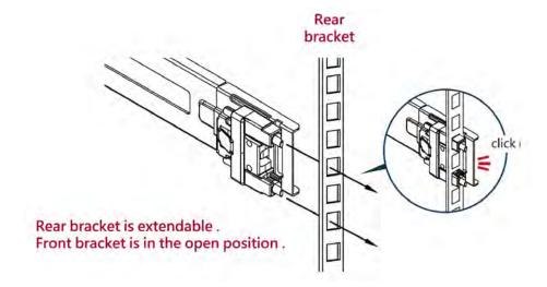
Step 4: Release the locking latch upward.
