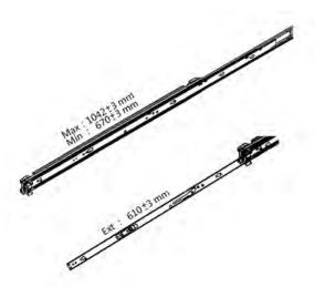
Step 1: Remove inner member. Pull inner member out as in the illustration.
