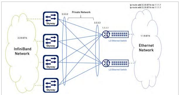
In this above use case, every Skyway-facing port on the side of the L2 Ethernet switches should be configured as a router port. In addition, a private network should be established (in the example above, 3.3.0.0/16) between the router ports mentioned above and the Skyways Ethernet port channel.
