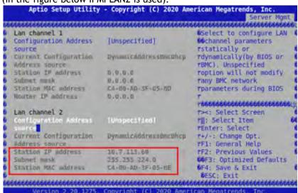
▲ "Lan channel 1" refers to IPMI LAN 1 and "Lan channel 2" refers to IPMI LAN 2.
