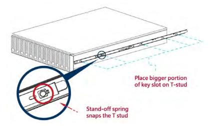
Step 3: Mount the cabinet member to the posts. Align the positioning pin to the desired complete U location, and pull the bracket forwards to lock it to the post. The bracket is locked to the post after a "click" sound is heard.
