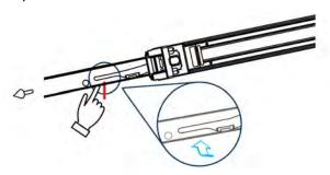
Step 2: Mount the inner member onto the chassis. Place the key slot on T stud, and push the inner member toward the back.
